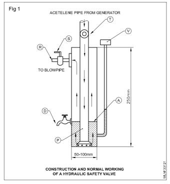
The pipe (P) has a baffle plate fixed at its lower end.
