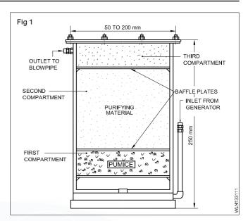
The first compartment contains pumice stone which absorbs moisture from the acetylene. The second compartment contains purifying chemicals, which remove sulphuretted and phosphorated hydrogen. The third compartment contains filter wool, which filters the lime dust and other foreign materials. Ammonia is removed within the generator when the gas passes through the water.
