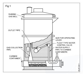
**Working principle:** Water is filled in the outer vessel through the water filling pipe and the water tap is turned off when there is sufficient water.
