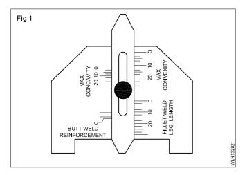
1 Leg size of fillet weld: To determine the fillet weld leg size the slot is placed against the toe of the weld as shown in (Fig 2)
