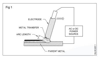
**Medium, normal arc** (Fig 2): The correct arc length or normal arc length is approximately equal to the diameter of the core wire of the electrode.
