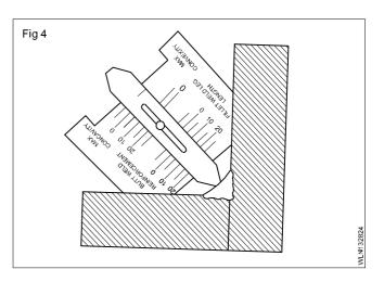
4 Acceptable reinforcement height on butt weld: To determine the acceptable size of reinforcement height on butt weld, the spoke portion of the gauge, flat portion may be scatted on either size of butt weld as shown in Fig 5, on sliding the pointer blade downwards so as to touch the reinforcement placed on the butt weld.
