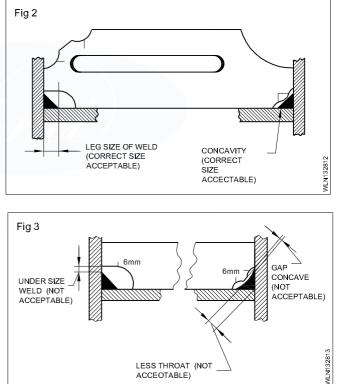
The gauges consist of struck which can be suitably altered according to the position of the used bead for fillet used butt weld.
