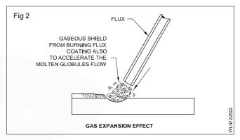
These gases expand and gain velocity. The flux sleeve direct these gases to flow in the direction of the molten metal. The gases flowing from the tip of the electrode have a pushing effect. Thus the metal globules are carried deep into the weld pool and influence penetration.
