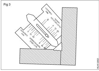
**3** Acceptable size of convexity: To determine the acceptable size of convexity the stock portion of the gauge having 45° angle sides touching both the members of the joints is placed as shown in Fig 4.
