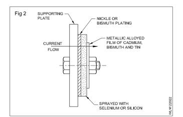
**Working principle:** The output of the step down transformer is connected to the rectifier unit, which converts AC to DC. The DC output is connected to positive and negative terminals, from where it is taken for welding purposes through welding cables. It can be designed to provide either AC or DC welding supply by operating a switch provided on the machine.
