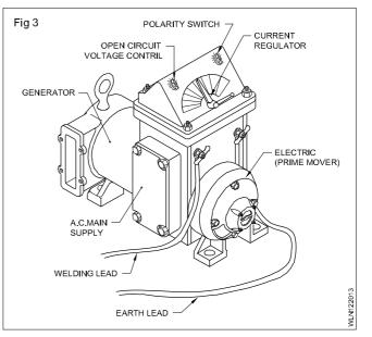
**Working principle of DC welding generator:** The armature is made to rotate with the help of a prime mover between the main poles, where a strong magnetic field exists
