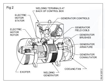
**Main poles:** These are connected to the body or yoke to produce magnetic lines of force, also called FIELD COILS.
