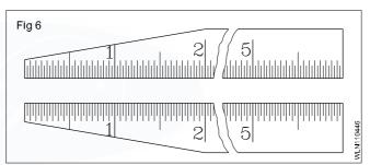
**Steel rule with tapered end:** This rule is a favorite with all mechanics since its tapered end permits measuring of inside size of small holes, narrow sots, grooves, recesses etc. This rule has a taper from 1/2 inch width at the 2 inch graduation to 1/8 inch width at the end. (Fig 6)
