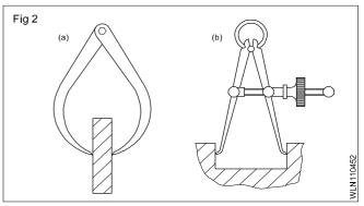
Calipers are used along with steel rules, and the accuracy is limited to 0.5 mm; Parallelism of jobs etc. can be checked with higher accuracy by using calipers with sensitive feel.
