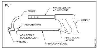
**Types of hacksaw frames:** The two different types of hacksaw frames are solid frames and adjustable frames.
