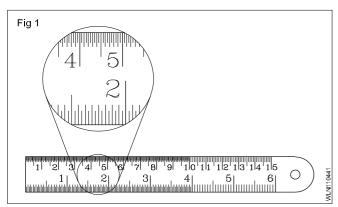
Steel rules are made of spring steel or stainless steel. These rules are available in length 150mm, 300mm and 600mm. The reading accuracy of steel rule is 0.5 mm and 1/64 inch.
