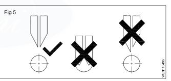
The divider point should be kept sharp in order to produce fine lines, frequent sharpening with an oilstone is better than sharpening by grinding. Sharpening by grinding will make the points soft.
