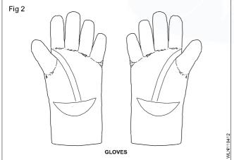
The leather apron, gloves, cape with sleeves and leg guard Fig 3,4,5 and 6 are used to protect the body, hands, arms, neck and chest of the welder from the heat radiation and hot spatters, from the arc and also from the hot slag particles flying from the weld joint during chipping off the solidified slag.
