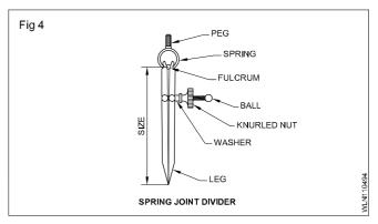
The two legs of the divider should always be of equal length. (Fig 5) Dividers are specified by the type of their joints and length.
