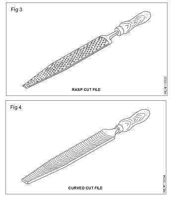
The selection of a file with a particular type of cut is based on the material to be filed. Single cut files are used for filing soft materials.
