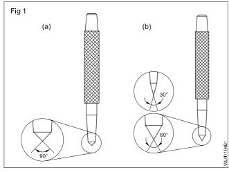
**Prick punch/Dot punch:** The angle of the prick punch is 30° or 60°. (Fig 1b) The 30° point punch is used for marking light punch marks needed to position dividers. The divider point will get a proper seating in the punch mark. The 60° punch is used for marking witness marks and called as dot punch (Fig 2)
